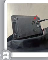
23 Plug the adapter into the corresponding hole of the control box. (See Figure 25)
