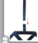
28 Insert and snap lock the base poles into the bases. (Watch J to J. See Figure 28)
