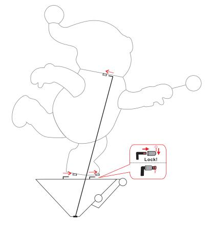
Install the metal support bracket to the back by inserting the rods into the loops first, then using the angled latch, lock the metal wire and support bracket.
