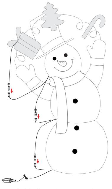
Connect the light plugs and connectors one by one as shown. Make sure all plugs are well connected. Using the transformer supplied, connect to a power source.
