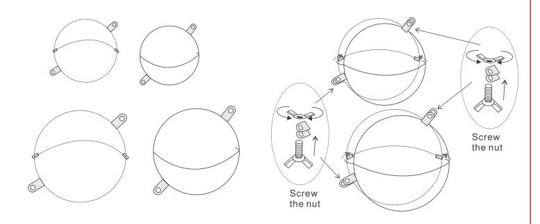
Assemble each ornament by inserting the screws through the holes and fastening with the wingnut provided.
