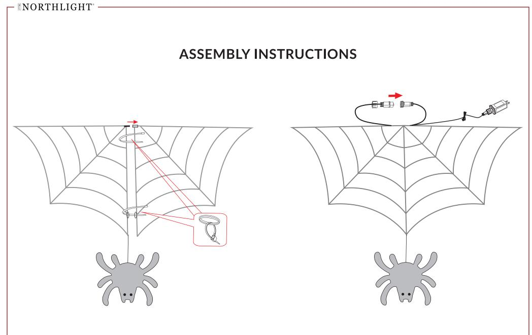
Attach the two web halves together by inserting the rod into the loop as shown above. Using the zip ties provided, tighten to secure. Connect the light plug and connector as shown. Make sure they are well connected. Using the transformer supplied, connect to a power source.
