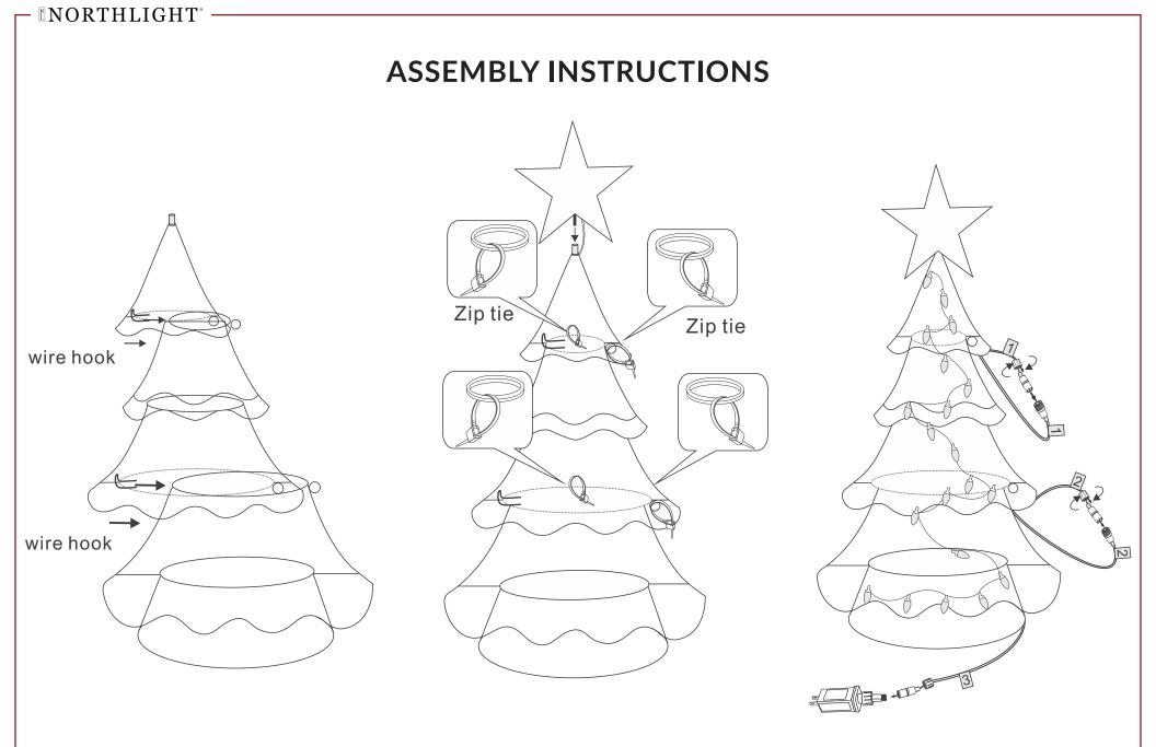
Insert the star to the top inserting the wire hooks as shown. of the tree as shown. Use the supplied zip ties to secure.
