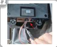
Plug the Try Me button into the corresponding hole of the control box. (See Figure 22)
