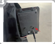
Plug the adapter into the corresponding hole of the control box. (See Figure 23)
