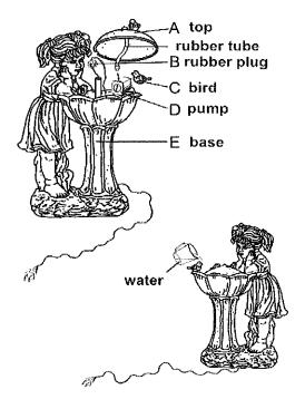
Step 1: Remove the product from the box; place E on the level surface.
